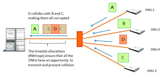
The GPON shared-network architecture makes the task of analyzing and pinpointing a rogue ONU challenging and extremely consuming in time and resources. The most common way to handle it is by turning off all the ONUs, and then turning them back on one-by-one until the faulty one is found. On top of being time-consuming, this process requires disconnection of traffic to every one of the customers on the PON. Needless to say, this is something that any service provider would like to avoid.
