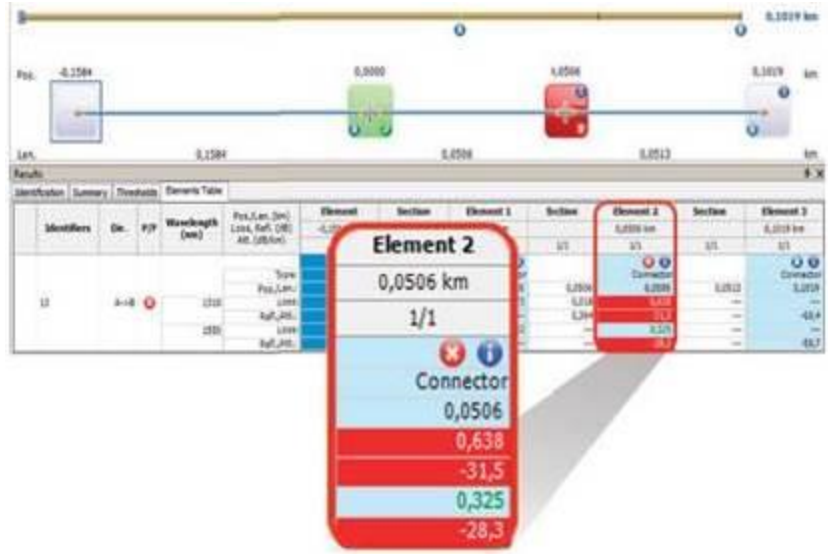
Figure 2. ORL and IL readings on an uncleaned connector.
