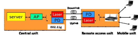
Fig. 4. Model of hybrid link IEEE802.11g WLAN-over-Fiber [5].
